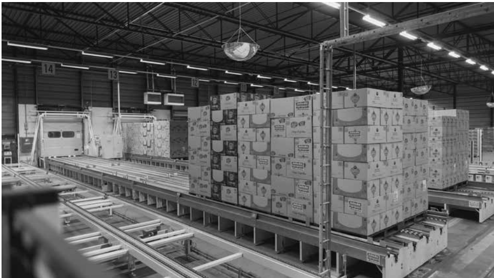
Figure 22.2 Pallets on a conveyor system, ready for automated loading/unloading
