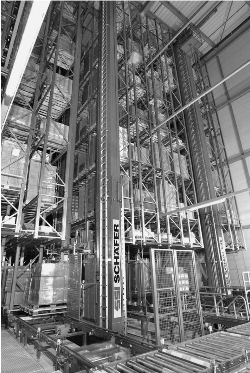
Figure 19.11 AS/RS crane, double-deep installation
