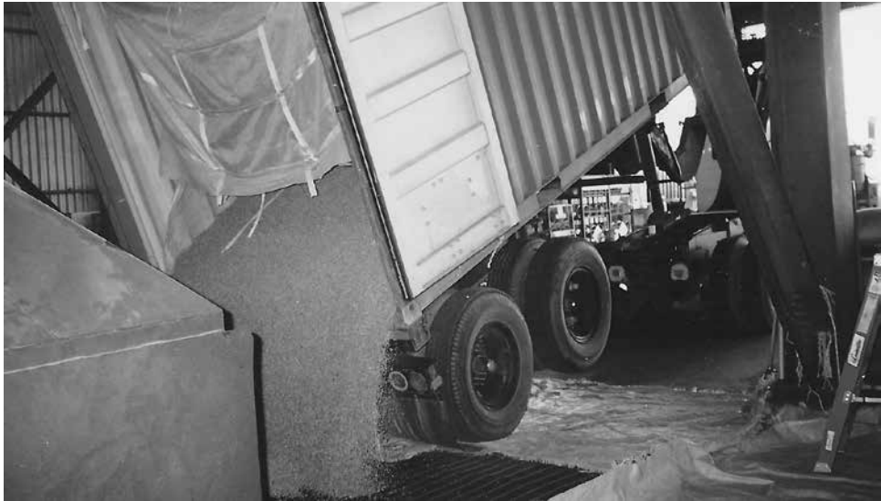
Figure 28.12 A container loaded with grain being unloaded by using a hydraulic ram to lift the trailer. The liner used to secure the grain inside the container can be clearly seen
