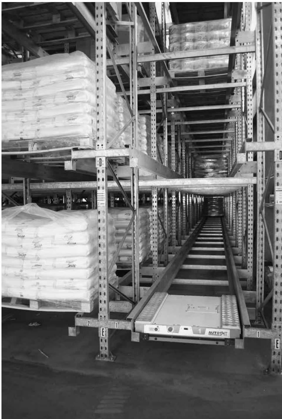
Figure 19.6 Shuttle racking, showing a pallet shuttle placed in the first rack position at low level
