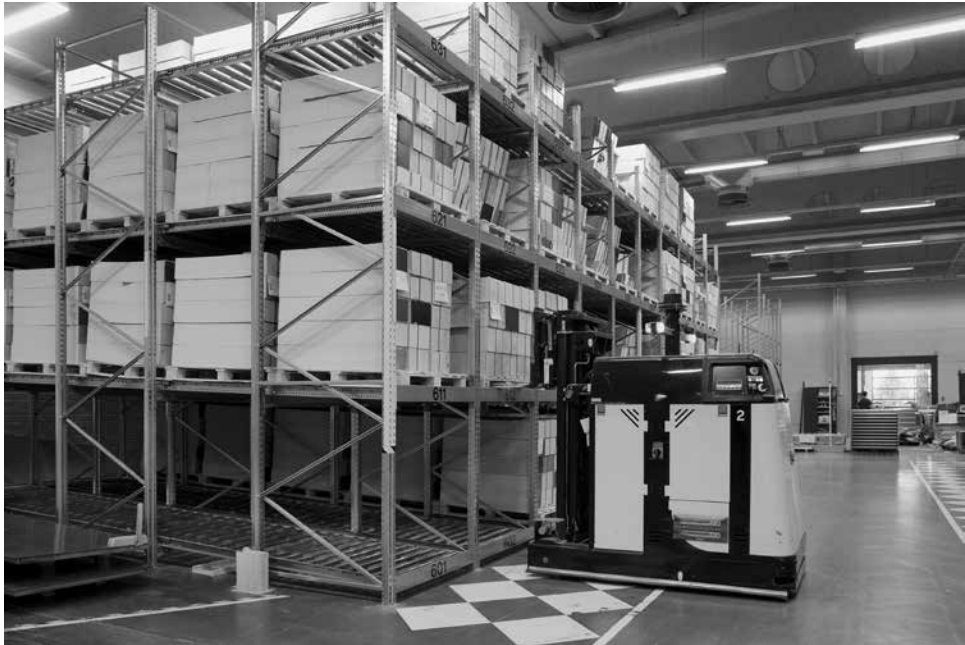
Figure 19.4 Robotic fork-lift truck serving push-back roller racking
