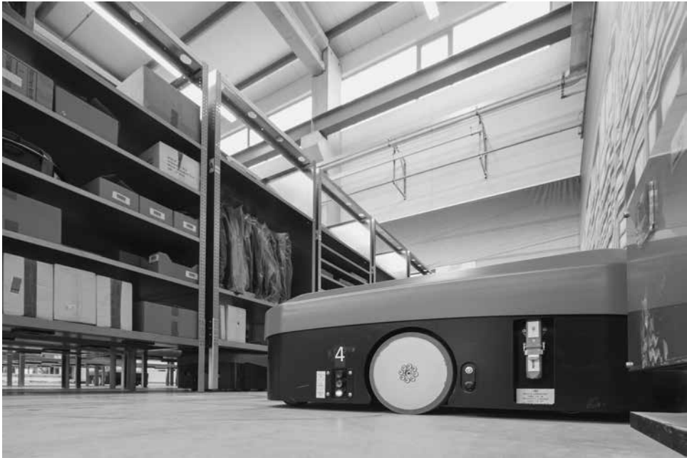
Figure 21.5 Shelf modules-to-picker system showing robotic drive units
