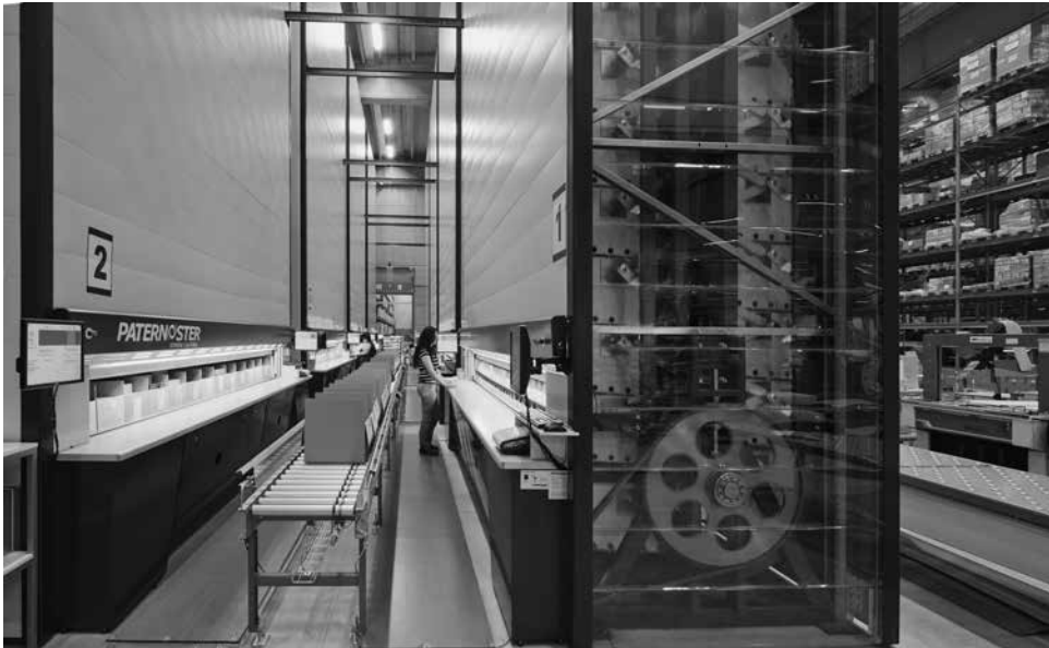
Figure 20.5 Vertical carousel showing the shelf rotation mechanism
