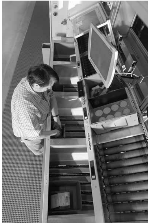
Figure 21.4 Totes-to-picker system with pick by light
